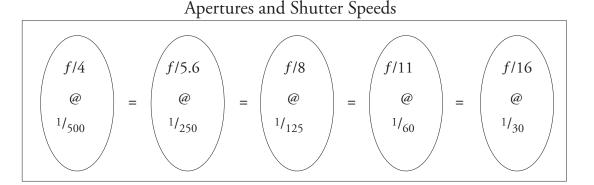
Note that the reason that each pair is equivalent to every other pair is that each shutter or aperture number lets in either one half as much or twice as much light as the number next to it. So, f/11 lets in half as much as f/8;  $1/_{60}$  of a second lets in twice as much light as  $1/_{125}$  of a second. It is a relationship of 1:2; twice as much or half as much.
